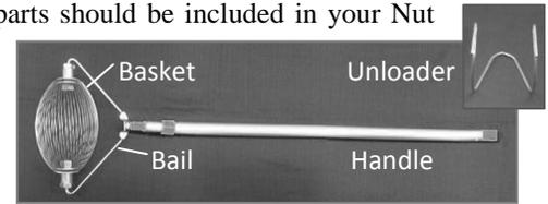
**Put the tool together.** The bail (shaped like a coat hanger) holds the basket so it can roll. Place the basket into one end of the bail, and then the other. Screw the bail into the handle until they are flush. If needed, add a washer to keep a tight fit.
